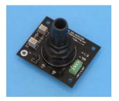
The PRECISION SOS DETECTOR™ is the first commercially available Start-Of-Scan detector made for the challenging environment inside a high power Polygon Scan Head. It is designed to work with the PRECISION SOS LASER DIODE MODULE™
