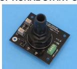
An SOS detector is required to achieve accurate line to line registration with any polygon scanner. It is used to synchronize a CW or pulsed laser to the scanner. (Galvo scanners need absolute encoders, polygon scanners need Start-Of-Scan detection.) Read more about it here:
